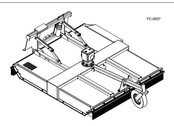
The SM72 rotary mower is designed to be operated on skid steer power units. These rugged Mowers are designed for medium-duty work and are related to cut vegetation up to 2" in diameter.
